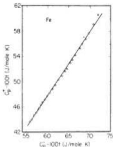
FIG. 3. Plot of interpolated specific heat,  $\tilde{C}_p^*$ , of iron for  $T > T_c$  as a function of actual  $\tilde{C}_p^*$  data for  $T < T_c$  at equal values of  $|t|$  after the linear lattice background has been subtracted off. The linear relation  $\tilde{C}_p^* = (-14.42 \pm 0.97) + (1.036 \pm 0.015) \tilde{C}_p^*$  shows strong evidence for the scaling law  $\alpha = \alpha'$ .
