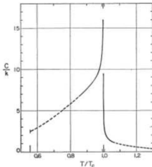
FIG. 1. Configurational specific heat of argon at constant critical density from the triple point to beyond the critical point. (The range of temperature marked on the axis close to  $T/T_c=1$  is shown in detail in Fig. 2.)
