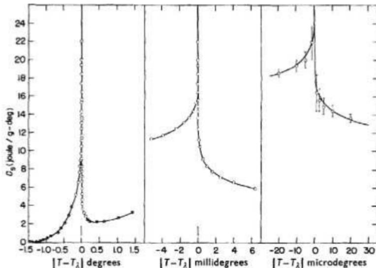
Fig. 2. Specific heat of liquid helium vs  $T - T_\lambda$  in  $^\circ\text{K}$ .
