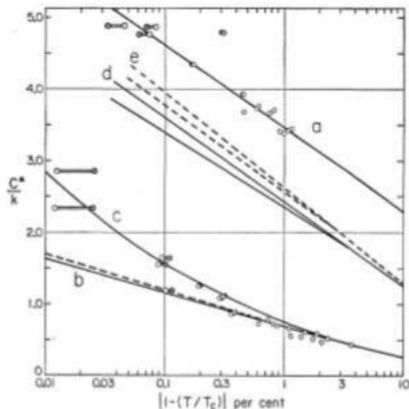
FIG. 3. Logarithmic plot of the specific-heat density  $C^*(T)$  for argon [experimental points and curve (a)], and for lattice gas models; (b) above  $T_c$  assuming a logarithmic singularity (solid line fcc, dashed line s.c.); (c) above  $T_c$  assuming  $\alpha=0.20$  (fcc); (d) below  $T_c$  for the fcc lattice; (e) below  $T_c$  for the s.c. lattice.
