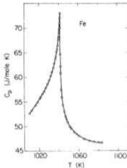
FIG. 2. Specific heat of iron plotted as a function of temperature.
